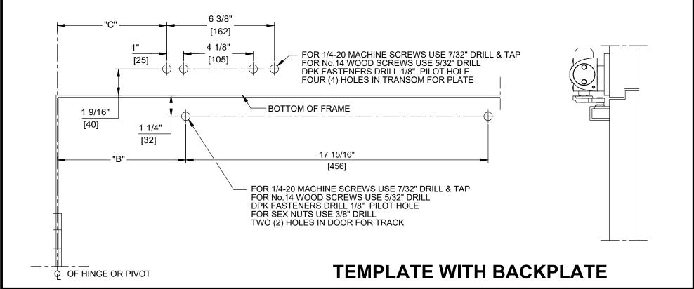
DOOR CLOSER MODELS: 7436 FT, FTH FLUSH TRANSOM TRACK INSTALLATION (PUSH SIDE MOUNT) WITH PLATES BP74T, BP86T, BP86TFC
